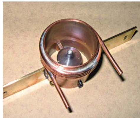
The polished aluminum occulter in its water-cooled copper housing
