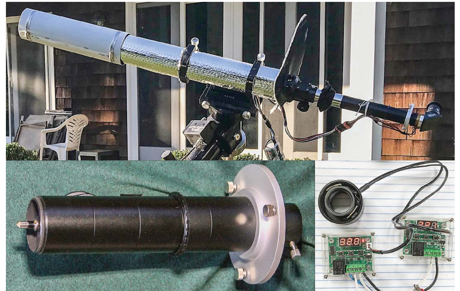
Figure 2: Hripcsak's telescope, the modified Baader prominence viewer with the cone exposed, and the homemade oven for the 530.3 nm filter.
