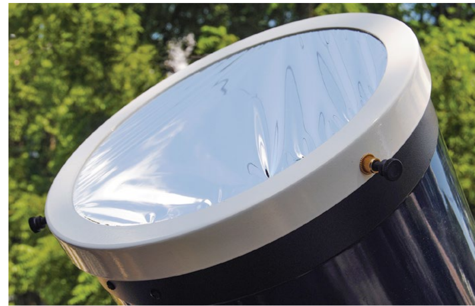
Figure 2. Pre-mounted Baader visual filter attached to a 10-inch Schmidt-Cassegrain telescope; nylon screws hold the filter securely in place.
