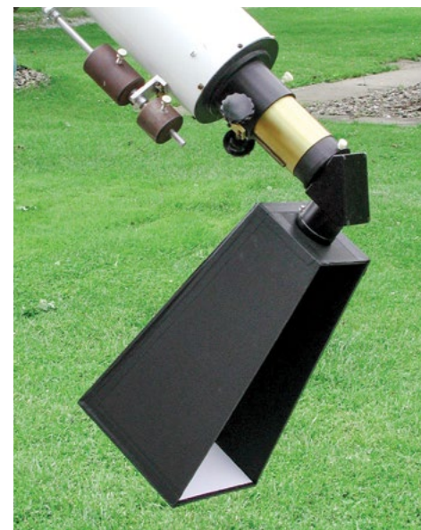
Figure 1. Hossfeld Pyramid constructed of black foam board with a Bristol board projection screen. When used in this position, with a star diagonal, the screen is always in the shade, permitting bright, contrasty views of the Sun.
