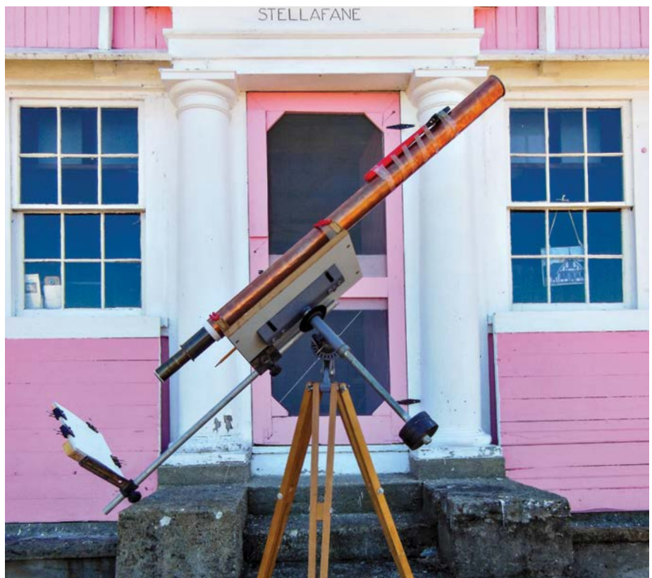
This simple homemade single-element refractor with a $5 objective purchased from Surplus Shed was one of three telescopes used by members of the Antique Telescope Society to collect simple sunspot data. The project allowed specialist Dr. Leif Svalgaard to propose a significant correction in the interpretation of eighteenth-century sunspot records. As solar activity now increases, additional observers are especially welcome in the project. Photo at the Stellafane Clubhouse by J. W. Briggs.
