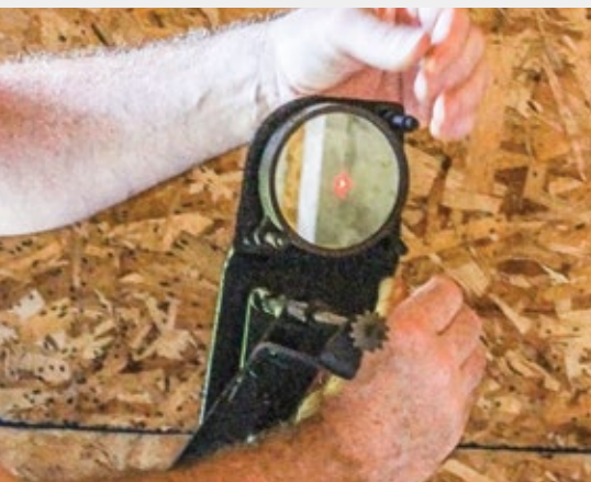
A laser aided in alignment of the mirrors. With 5 reflections in the system, alignment is a painstaking process. This must have been a much more difficult task before lasers! Photo by Michael Patterson.
