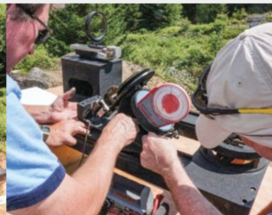
Dave Groski and Matt Considine aligning the polar axis of the clock-driven coelostat mirror in 2016. This mirror reflects the Sun to the steering mirror, which directs the beam into the observatory. Photo by Michael Patterson.
