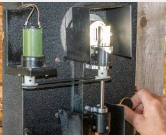
A solar image focused on the input slit. Note the rotating prism in front of the slit, which scans the image across the slit. A second prism on the same shaft (out of frame) reconstructs the image after the exit slit. Photo by Michael Patterson.
