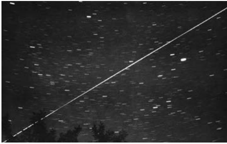
Figure 1: Echo I Satellite July 21, 1962 11:50 pm EST. Kodak Tri-X film 5-minute exposure with a Brownie Hawkeye Camera (45 mm f/2.8 lens). Echo I was a 100-foot diameter reflective Mylar balloon in an approximate 1500 km high orbit.
