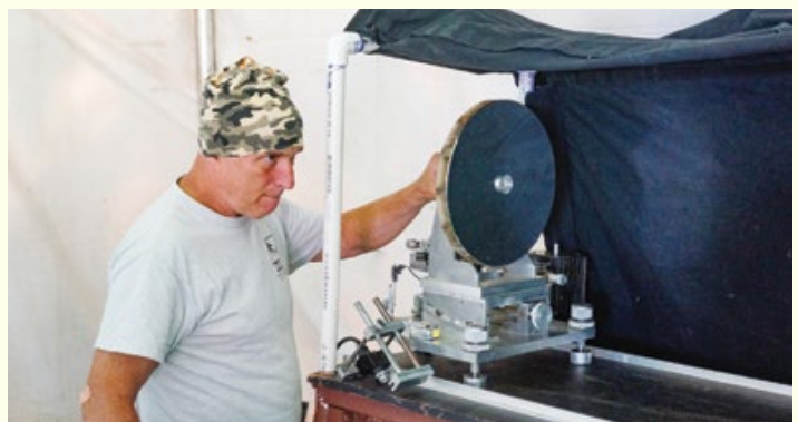
Dave Kelley preparing to test a mirror with his autocollimation flat. Photo by Doug Arion.
