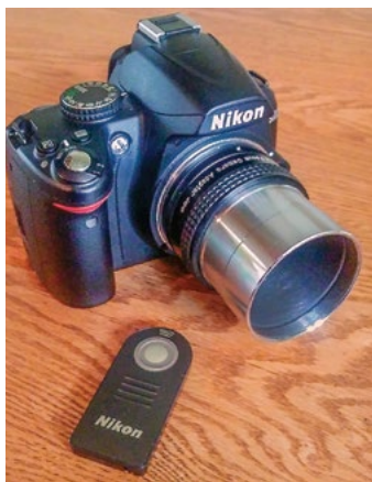
Nikon D3000 DSLR with T-ring and 2-inch focuser adapter. Button device in foreground is for remote hands-off shutter activation.
