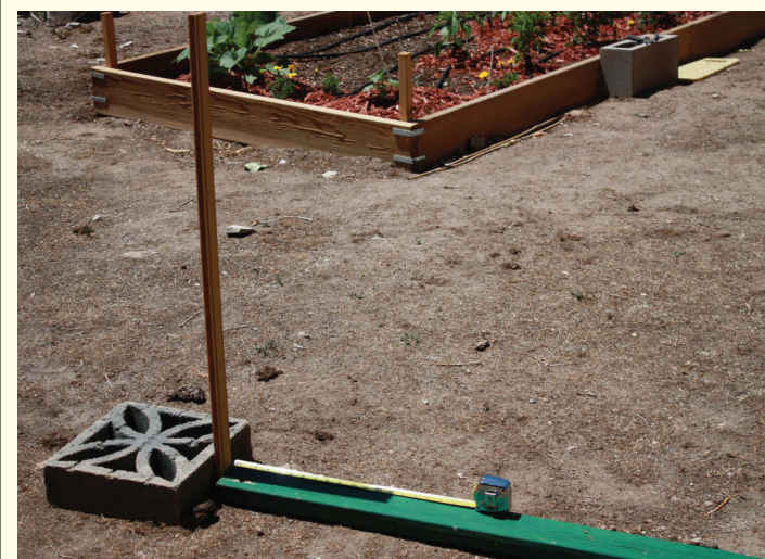
Figure 2: My "high-tech" setup to measure the Sun's shadow. The concrete block is to prevent movement due to the famous Pueblo West winds.
