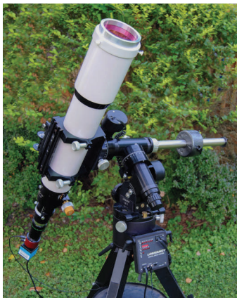
Author’s 102 mm f/7 Megrez (William Optics) telescope fitted for H-alpha solar observing and imaging. On the objective end is a Lunt 100 mm energy rejection filter, at the eye end a 2x Tele Vue Powermate, Daystar Quark chromosphere filter, and an Imaging Source DMK 41AU02 video camera.
