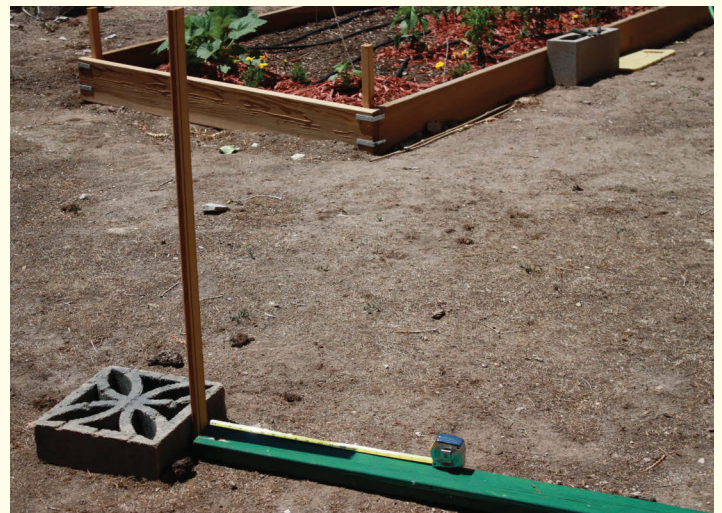
Figure 2: My “high-tech” setup to measure the Sun’s shadow. The concrete block is to prevent movement due to the famous Pueblo West winds.
