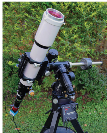
Author’s 102 mm f/7 Megrez (William Optics) telescope fitted for H-alpha solar observing and imaging. On the objective end is a Lunt 100 mm energy rejection filter, at the eye end a 2x Tele Vue Powermate, Daystar Quark chromosphere filter, and an Imaging Source DMK 41AU02 video camera.
